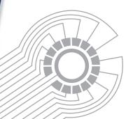
**Circuit:** 16 Position Selection Attributes: Used in those applications that require a single switch closure at each detent position. Positions can range from 2-24 (16 position shown) **Example:** Motor Speed Control
