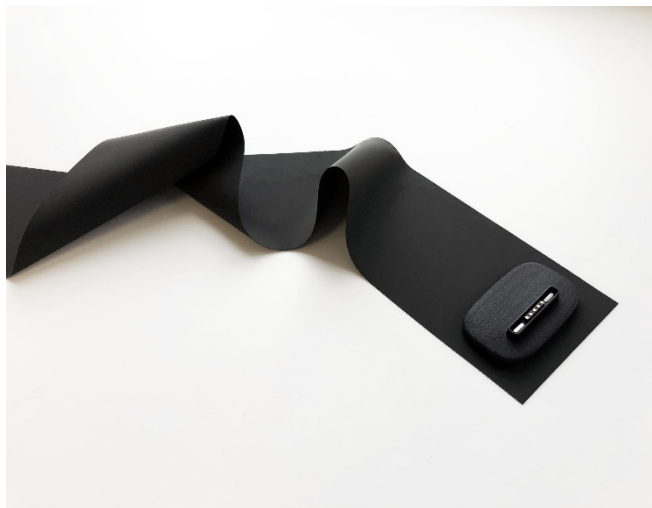
A power and data line within the LOOMIA Electronic Layer can support sensors and power transmission.
